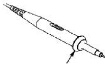
Figure 3-8: Finger Safety Ring of the Probe
