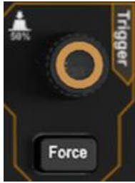
Figure 5-1: Trigger control area
