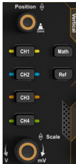
Figure 5-4: Vertical control area
