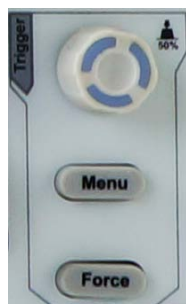
Figure 3-13 Trigger Control Zone
