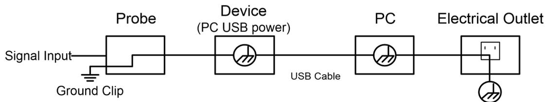
It is NOT allowed to measure AC power when the device been powered by AC power source through the adapter, or when the device powered by by PC through USB connection cable (via USB communication interface of PC, with PC powered by AC power source)..
