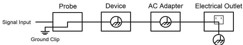
When the device communicating with PC via USB communication interface (with PC powered by AC power source), the illustration of the ground wire connection -
