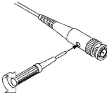
Figure 3-7 Adjust Probe
