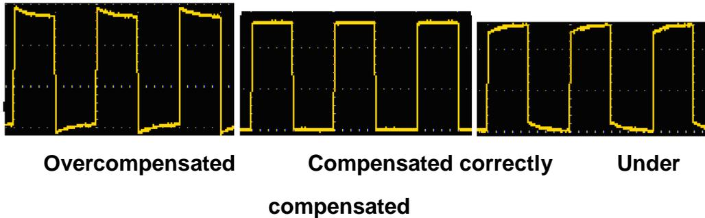
Figure 3-6 Displayed Waveforms of the Probe Compensation
