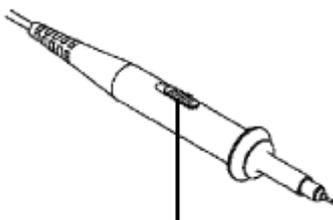
Figure 3-8 Attenuation Switch
